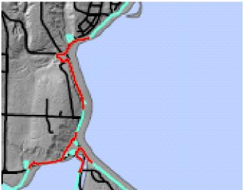
The figure shows where estimated sea level elevations (blue lines) intersect the road surface elevation.
